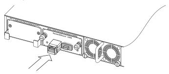
Figure 5: Installed QSFP+ Module (Summit family switch and BlackDiamond 8800 series switch)
